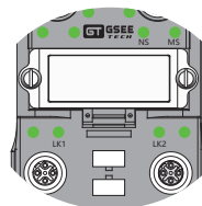
M12 D-Code, ETHERNET/IP Link 1/2 接线示意
