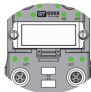
M12 D-Code, ETHERNET/IP Link 1/2 接线示意
